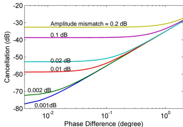
Figure 2: Theoretical cancellation vs. precision in amplitude and phase matching.
