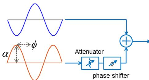
Figure 1: Operating principle of active interference cancellation.
